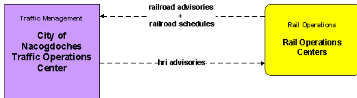
Figure A56 – ATMS15 – Railroad Operations Coordination: City of Nacogdoches Traffic Operations Center
